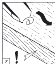
7 WHEN WORKING ALONG THE GRAIN BE AWARE OF SUDDEN DOWNWARD GRAIN DIRECTION
